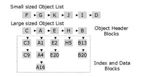
Fig. 3 SOL (Small sized Object List) and LOL (Large sized Object List).
